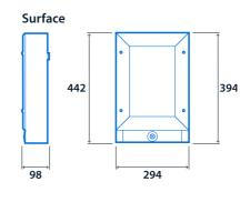
Minimum cut-out - 270 x 420 Maximum cut-out - 600 x 600
